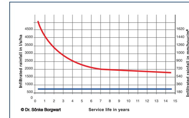
American and German experience recommends that the design infiltration rate through the surface should be 10% of the initial rate, to take into account the effect of clogging over a 20-year design life without maintenance. Even after allowing for clogging, studies have shown that the long-term infiltration capability of permeable pavements will normally substantially exceed UK hydrological requirements (for example, an extreme storm of 100mm/hour as shown blue in the graph).
