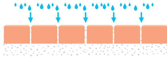
The key to CBPP is its permeable surface zone of high-strength concrete blocks with angular aggregate (2/6.3mm) used to fill enlarged joints and as a laying course.
