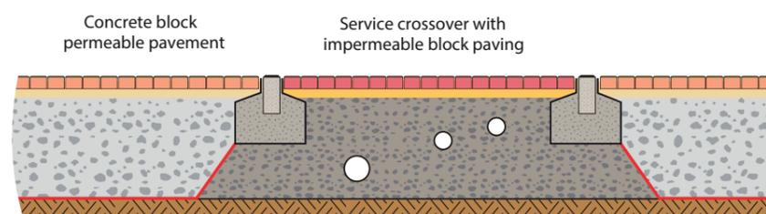
Cross section through impermeable paving service corridor.
