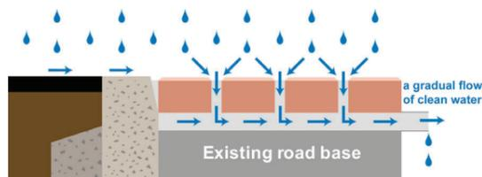
The same blocks and 2/6.3mm grit bedding layer and jointing material as for permeable pavements generally are used. Water is attenuated, treated and conveyed within the laying course, which is key to this technology, enabling filtration of silt and retention/treatment of pollutants without clogging.
