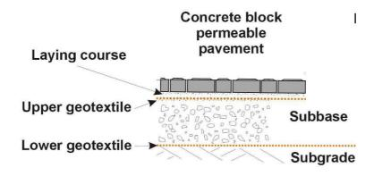
Figure 1 Geotextiles in a permeable pavement
