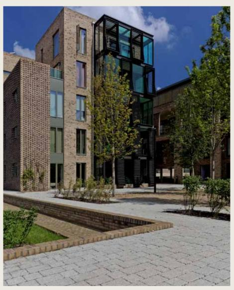
Sparkling granite finish concrete block permeable paving helps to characterise the 'Great Court'
