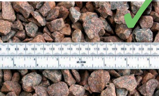
Typical permeable sub-base aggregate has voids between for water.
