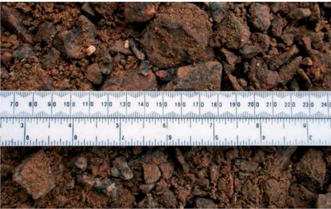
**Permeable pavement sub-base aggregate** – Crushed rock or similar material that does not have fine material in the spaces between rock pieces, allowing water to flow easily through the voids. Proprietary coarse graded aggregates specifically for permeable paving are available from many suppliers.
