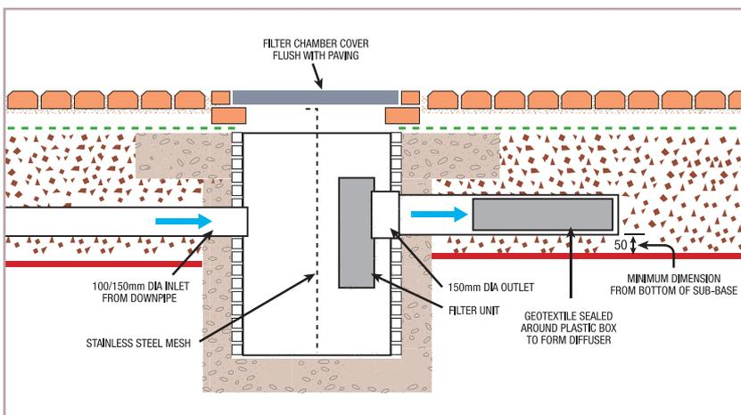
Roof water is piped into filter chambers which remove rubbish and silt, then dissipated through diffuser boxes into the permeable sub-base under the CBPP.
