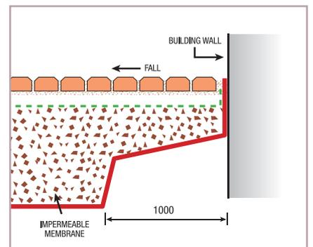
Concrete block permeable paving runs right up to the school building but the permeable sub-base is curtailed 1 metre away from the building with a clay protection to the foundation. Water is contained within the sub-base and provision made for excess storm water runoff so that it cannot enter the building.
