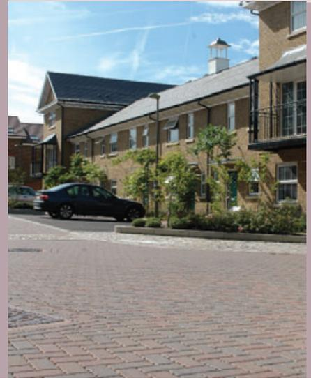
Concrete block permeable paving is a unique sustainable drainage system with important attenuation and pollution source control characteristics. It provides an attractive pavement surface suitable for trafficking that also acts as a drainage system. More information is available in *Understanding Permeable Paving* available on the Interpave website [www.paving.org.uk](http://www.paving.org.uk)
