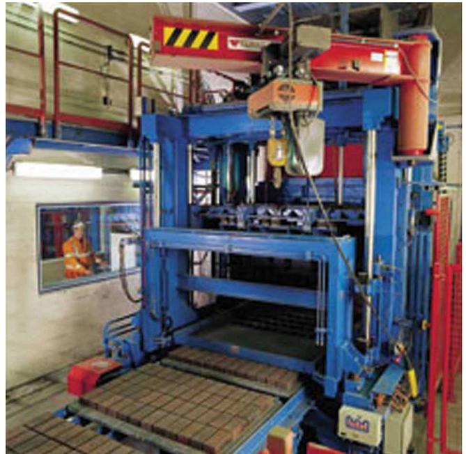
*Investment in state-of-the-art robotic equipment and related processes by one Interpave member avoids workers handling product and has reduced the lost time injury frequency rate by over 65%.*
