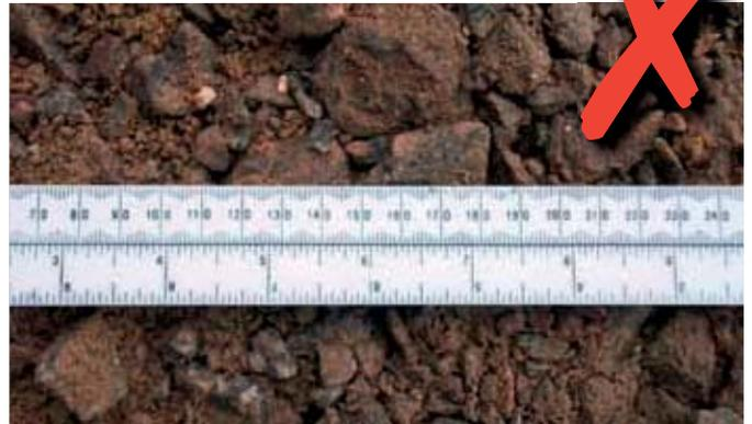
Type 1 aggregate for conventional block paving is not permeable when compacted.
