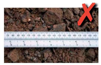
Type 1 aggregate for conventional block paving is not permeable when compacted.
