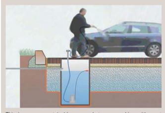
This is a more sustainable approach to car washing with most of the water automatically treated for reuse as it passes through the permeable paving.
