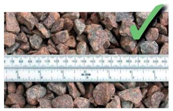
Typical permeable sub-base aggregate has voids between for water.
