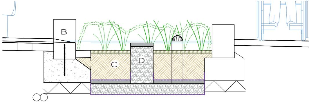
Strategically-placed, small bioretention raingardens accept polluted highway runoff through gaps<sup>B</sup> in granite kerbs. An innovative, two-tier approach was applied to bioretention design, incorporating a particular soil blend (known as 'RBA SuDS Soil'). This approach responds to the pollution hierarchy of smaller rainfall events and the first flush of larger events, whilst ensuring healthy and resilient plant growth suitable for demanding urban environments.
