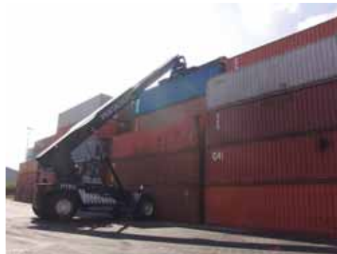
Figure 12. Reach Stacker handling 40ft container. Note how a fifth container can be accessed in the second row.
