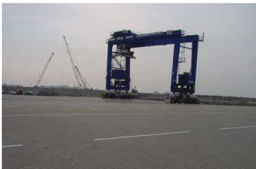
Figure 18. Rubber Tyred Gantry Crane (RTG). Individual wheel loads can exceed 50t. This machine has 16 wheels which reduces wheel load and thereby pavement thickness required.
