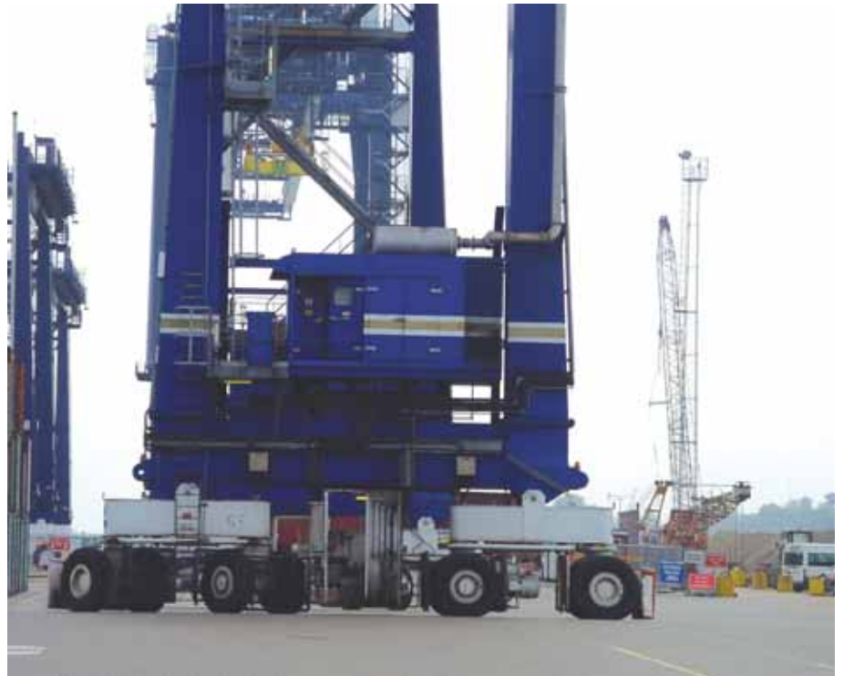
Figure 2. Some Rubber Tyred Gantry Cranes (RTGs) can turn their wheels through 90° whilst stationary. This can lead to surface instability.
