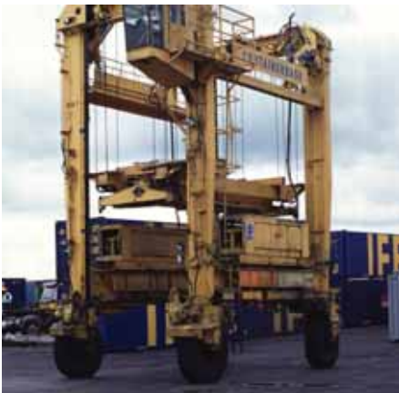
Figure 4. Four wheel straddle carriers apply wheel loads in excess of 20t.
