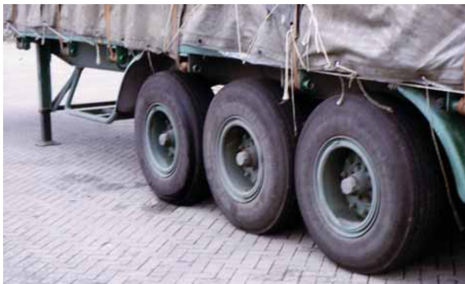
Figure 5. Highway trailers may have three axles, each applying 11t. The small steel plate may apply even greater load when the trailer is parked.
