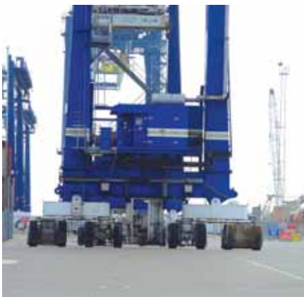
Figure 2. Some Rubber Tyred Gantry Cranes (RTGs) can turn their wheels through 90° whilst stationary. This can lead to surface instability.
