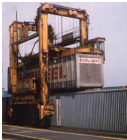
Figure 8. When operating within container stacks, a straddle carrier tracks the same length of the slab each pass.
