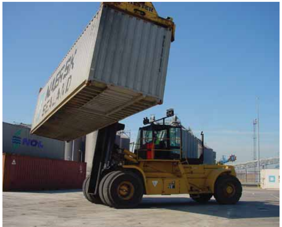
Figure 4. Four wheel straddle carriers apply wheel loads in excess of 20t.
