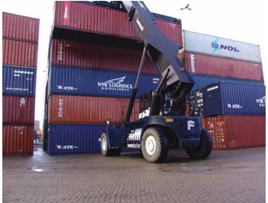
Figure 26. Reach Stacker operating in five high container stacks.
