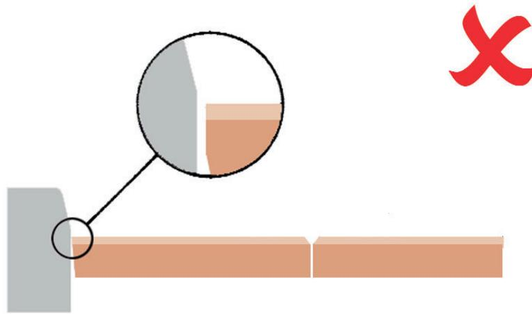
Cut faces should be positioned against an adjacent flag to reduce the visual intrusion of the square cut edge.
