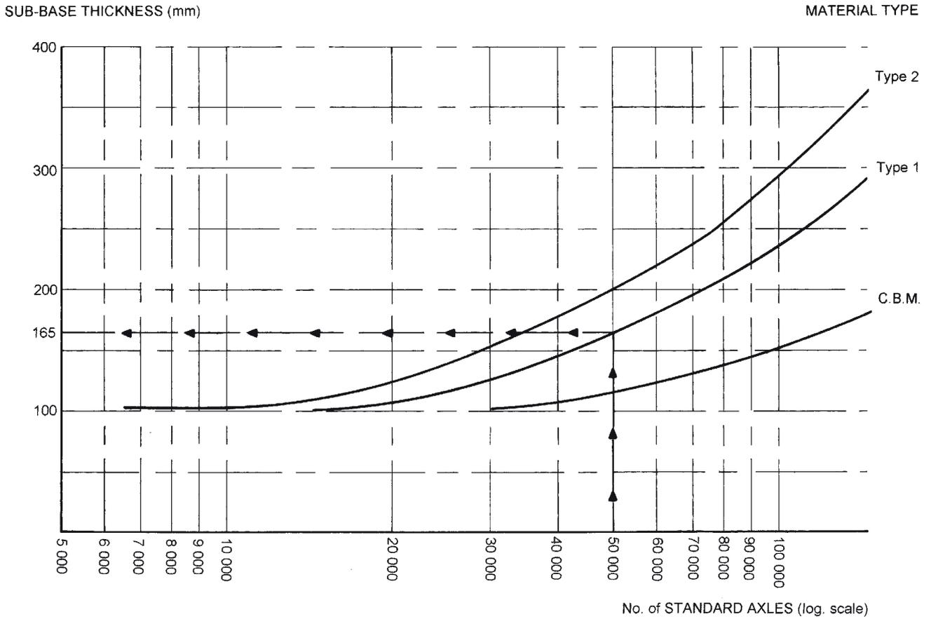
Graph 2; Sub-base thickness to prevent subgrade overstressing [Type E and Type F flags]
