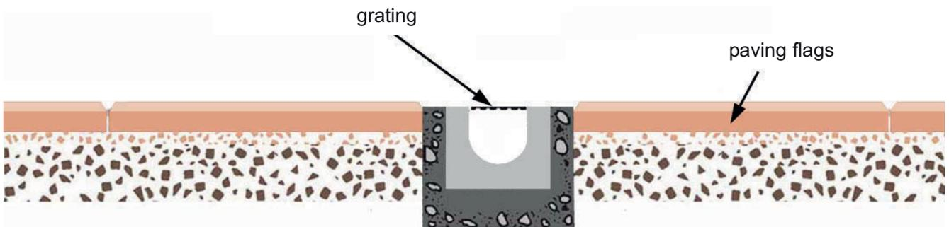
A ramped crossing may be formed in a flag footpath where the footpath and drive threshold are at similar levels. Two corner flags have to be cut to accommodate the change of level at the kerb.
