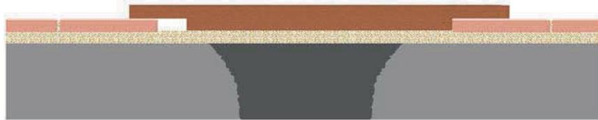
2. Use a rectangular steel float to hand screed areas that can't be screeded with the board
