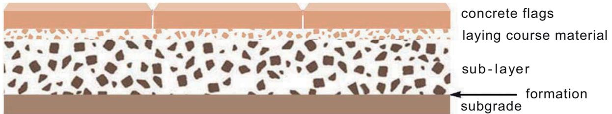
The fundamental objective is the assessment of the thickness of base material to be used beneath precast concrete flags to ensure that the allowable stresses in the paving units or sub-grade are not exceeded. The design of the pavement should be based on the assumptions that the construction conforms to BS 7533-4.
