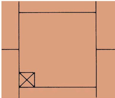
Where more than 25% of the flag has to be cut away then the remaining shape should be mitred from the internal corner of the cut-out to the external corner of the flag as shown below.
