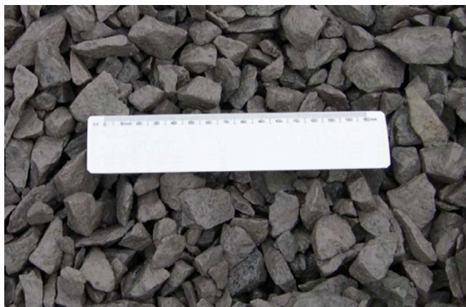
Figure 47: Typical 4/20 coarse graded aggregate sub-base
