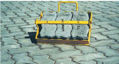
Figure 12. A sample panel of good, marginal, and unacceptable pavers used by factory and site personnel provided visual acceptance criteria of the paver surface texture. This was part of a comprehensive program of quality control and quality assurance measures implemented throughout the project.
