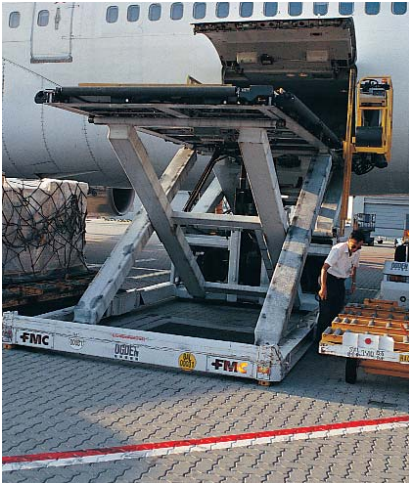
Figure 3. Steel stabilizer legs under cargo loading equipment concentrate point loads on pavements.
