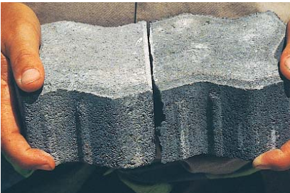
Figure 14. The left half shows a saw-cut paver with a chamfer on the cut edge. The right half shows a paver with rough edges cut with a manual splitter. No pavers at Hong Kong were cut with a splitter. Saw-cut pavers and chamfers eliminate risk of ingestion of chipped concrete into jet engines.
