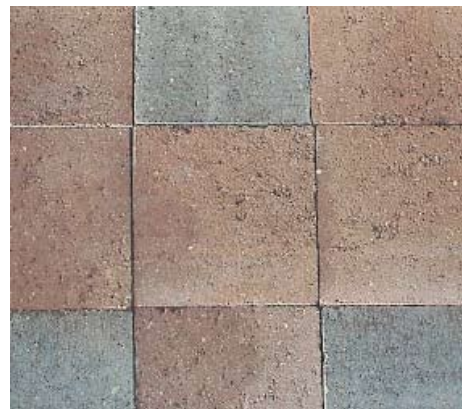
The same blocks after weathering
