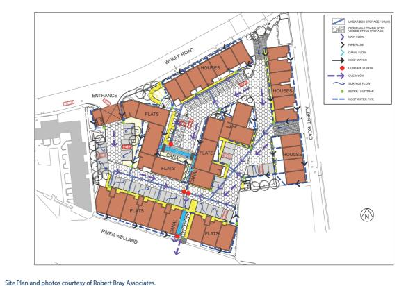
CBPP can help deliver SuDS on high-density urban developments, as well. At this 104-units per hectare town-centre housing scheme in Stamford, most public areas between buildings are CBPP which also accepts runoff from other hard areas and roofs. Stored, treated water then passes from the paving directly into planted rills and canals, which add interest and much-needed greenery to the courtyard environment, before passing into the nearby river.
