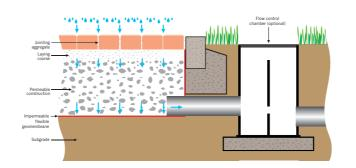
However, alternative structural layers are increasingly being used to cater for trees and green infrastructure, provide additional storage, accommodate statutory services or meet other requirements. The ability of CBPP to remove silt is particularly important to protect many of these alternative structural layer systems from clogging.
