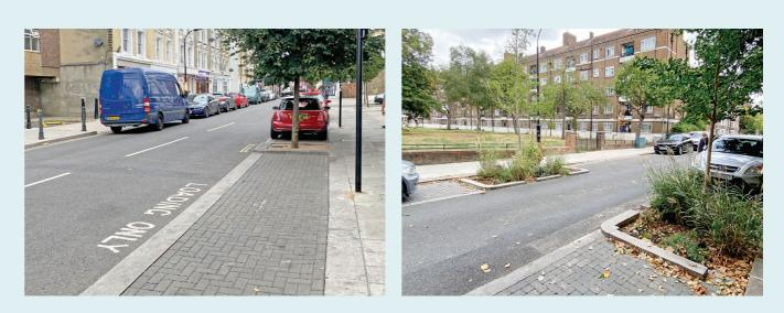
Two different profile examples of typical street enhancements in Hammersmith & Fulham, London (case study via www.mpaprecast. org), characterised by low-intervention CBPP on-street parking. As well as delivering SuDS and irrigation for trees, the puddle-free CBPP retains litter, silt and pollutants on the surface for removal with straightforward cleaning.
