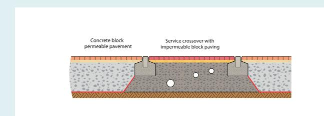
Cross section through impermeable paving service corridor.
