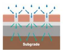
not sand. This arrangement ensures that water will continue to pass through the joints over the long-term.
