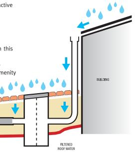
INFILTRATION FROM PERMEABLE PAVEMENTS
