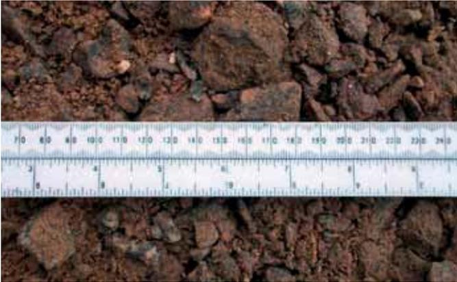
**Permeable pavement sub-base aggregate** – Crushed rock or similar material that does not have fine material in the spaces between rock pieces, allowing water to flow easily through the voids. Proprietary coarse graded aggregates specifically for permeable paving are available from many suppliers.
