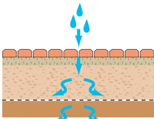
**Infiltrating** concrete block permeable paving
