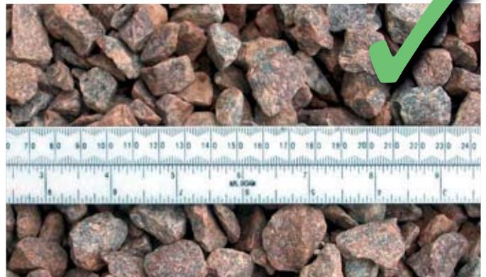
Typical permeable sub-base aggregate has voids between for water.
