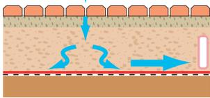
**Tanked** concrete block permeable paving
