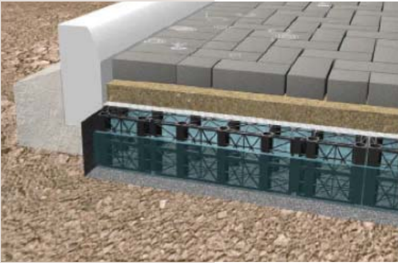
Figure 8: CBPP with geocellular sub-base replacement system below
