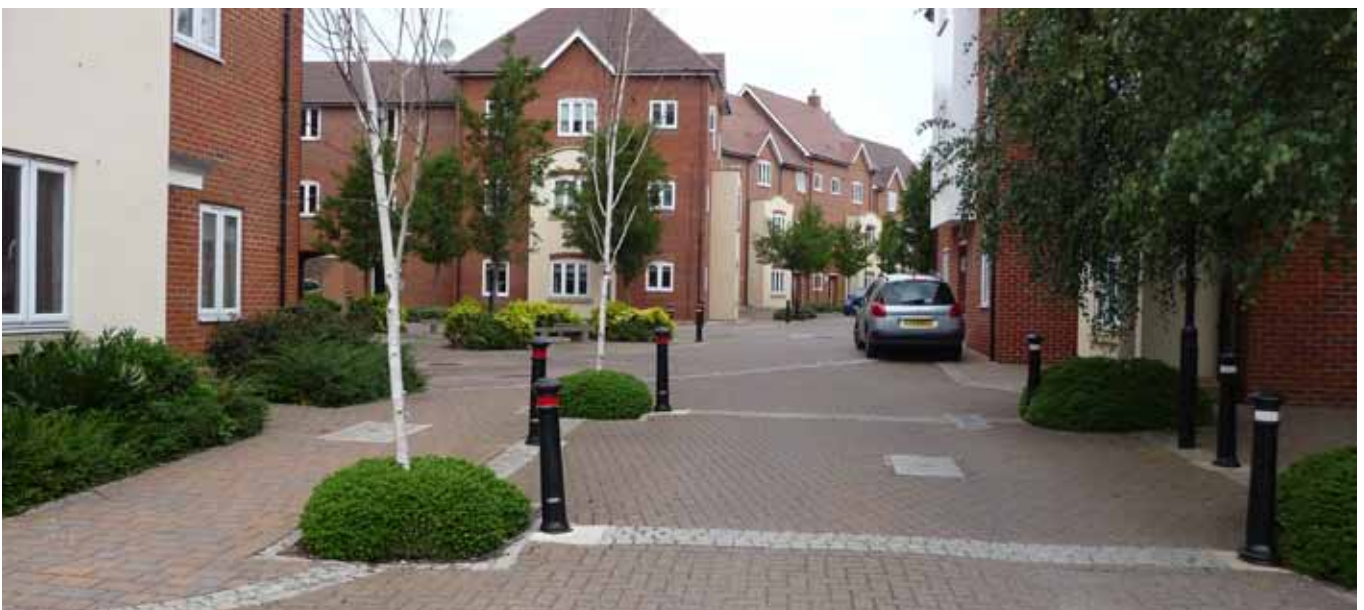
Penlon in Abingdon is a high-density housing scheme where space is at a premium. Here, concrete block permeable paving provides a lively, attractive surface, and sustainable drainage with no additional land-take.
