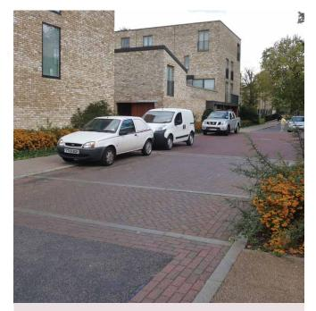
Block paving and concrete kerbs combine with resin bonded gravel and coloured macadam to give richness from a limited palette of paving materials. 2011
