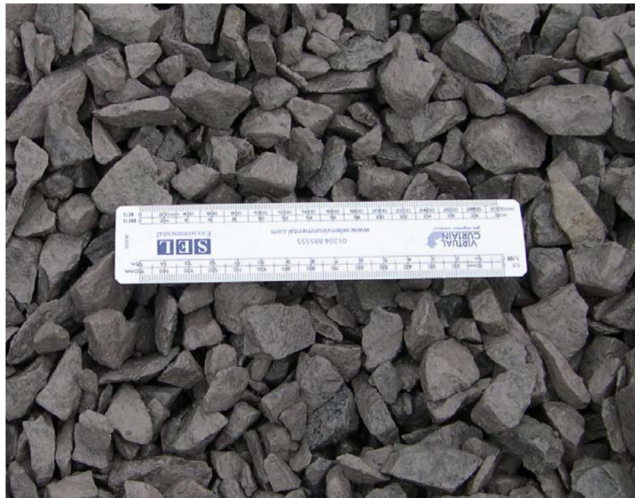
Figure 36: Typical 4/20 coarse graded aggregate sub-base material.
