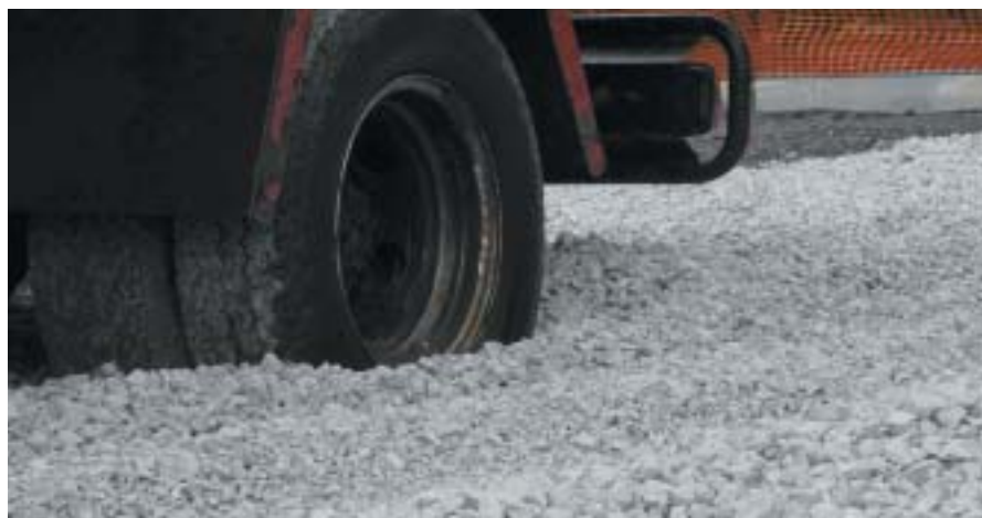
The truck used in the Martlesham trial became trapped in the clean stone after a few passes but the installation of CBPP created a stable pavement.
